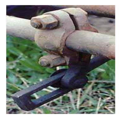
A close-up of a soldier and a slotted lock rod. A slotted lock rod was used when two (or more) rocking shafts drove one lock. This was common. In this case, two shafts drove a Main lock. When the soldier rotated (counter clockwise) the tail moved away from the camera and operated the lock rod. When the other soldier driving this lock rod rotated (not visible in this photo) the lock rod simply slid over the tail of this soldier.
